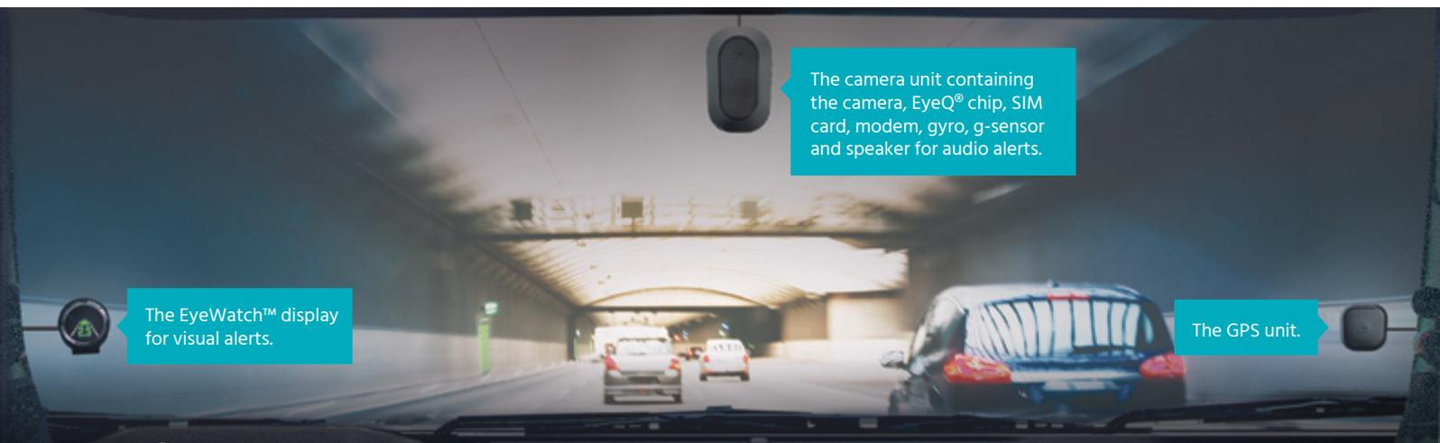
The camera unit containing the camera, EyeQ® chip, SIM card, modem, gyro, g-sensor and speaker for audio alerts.
